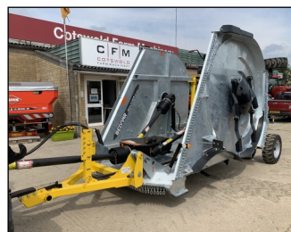
New Bednar MZ6000 mulcher/topper, 6m working width, 3m transport width, 1000 PTO speed, galvanized body. £17,450
